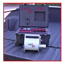
The industry leading S2S (Surface to Sandface) Logger provides accurate field readings (fluid level and surface pressure data) required for monitoring a producing well, calculating producing pressures (annular fluid depression test), or Buildup and Falloff tests for AER annual testing requirements. Buildup and Falloff test results can also be further analyzed for full pressure transient analysis of the reservoir.
